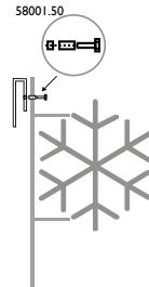
2. Fix the base from 58001.50 on a pole using metal strip 58005.50 and clips 58006.50.
