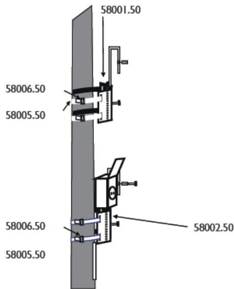
2. Fix the base from 58001.50 on a pole using metal banding tape 58005.50 and buckles 58006.50.
