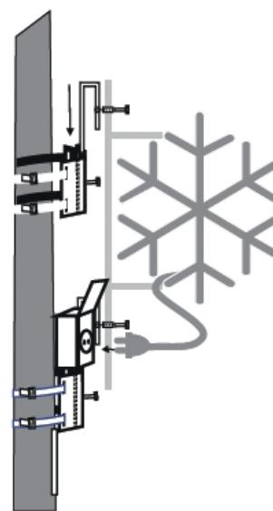
3. Assemble both parts of 58001.50, secure together and connect power cable to the power source.
